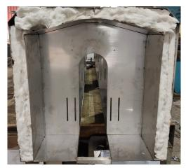
(5) 6 shrink sections, total 12 pcs of adjustable steam spray tubes are adjustable for complex shapes of bottles.
